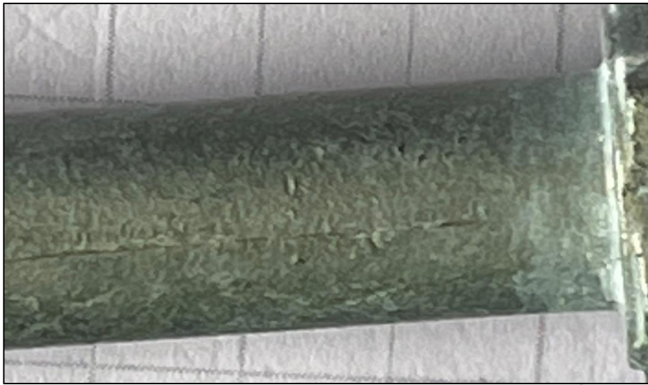
After 1000 Hours SST, No red rust spots, Tests Stopped
