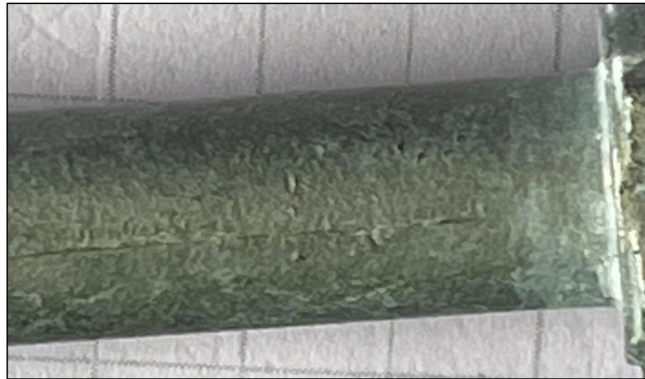
After 500 Hours SST, No red rust spots, Tests Stopped
